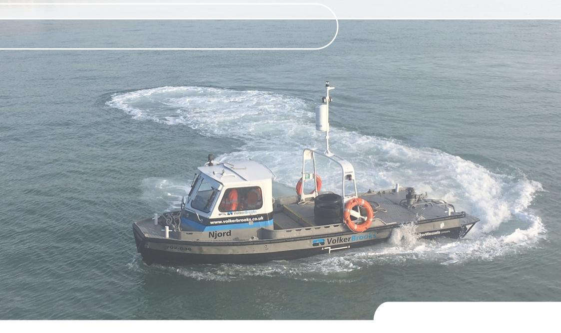
This vessel has been assessed as a Category 6 vessel, as defined within the MGN280 (with a one-mile restriction and only to be operated in favourable weather). Usually, it would be daylight only operations on this provision, however, the vessel may be used as above, but with a Category 3R restricted provision, if all safety equipment is on board to support this operation. Suitable risk assessments and method statements also need to have been completed.
